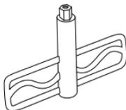
Lid with integrated pull mechanism
